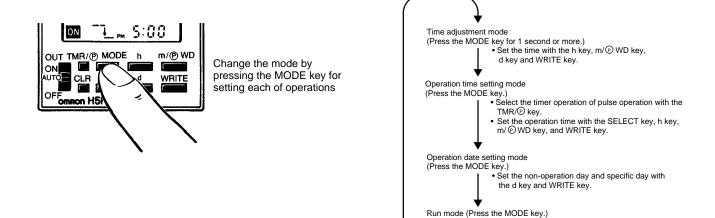
The time and date setting procedures in various operation modes are illustrated with display and key operation examples. (The shaded portion in the display indicates that indicator is blinking.)
